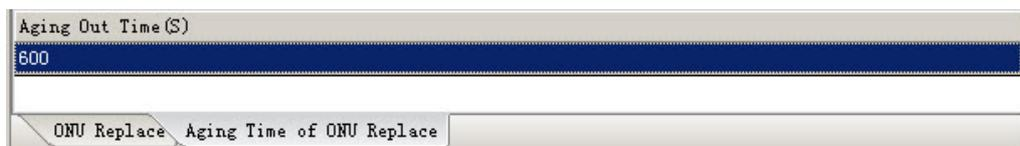
Figure 8-7 Configuring the replacement aging time of an EPON ONU
