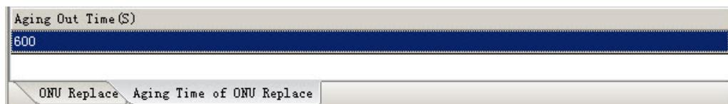
Figure 8-2 Configuring the replacement aging time of an EPON ONU
