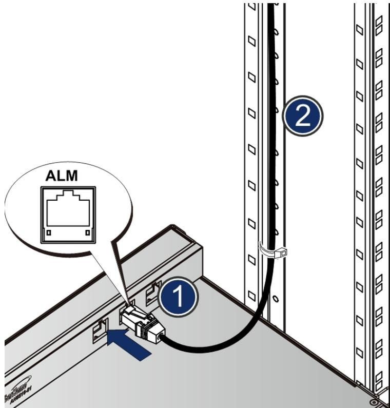
Figure 7-16 Arranging the alarm cable
