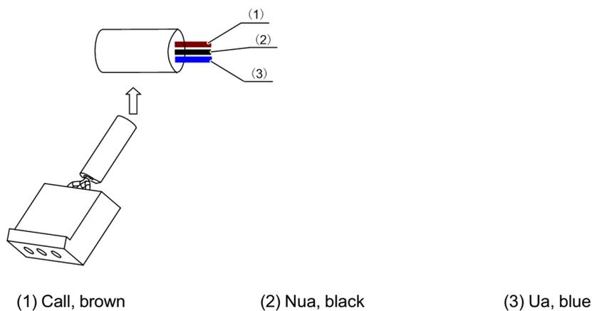
Figure 7-20 The alarm cable for the head of row cabinet
