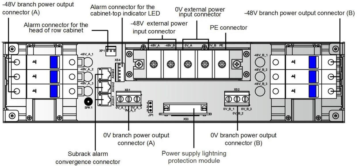
Figure A -2 The PDP's connectors
