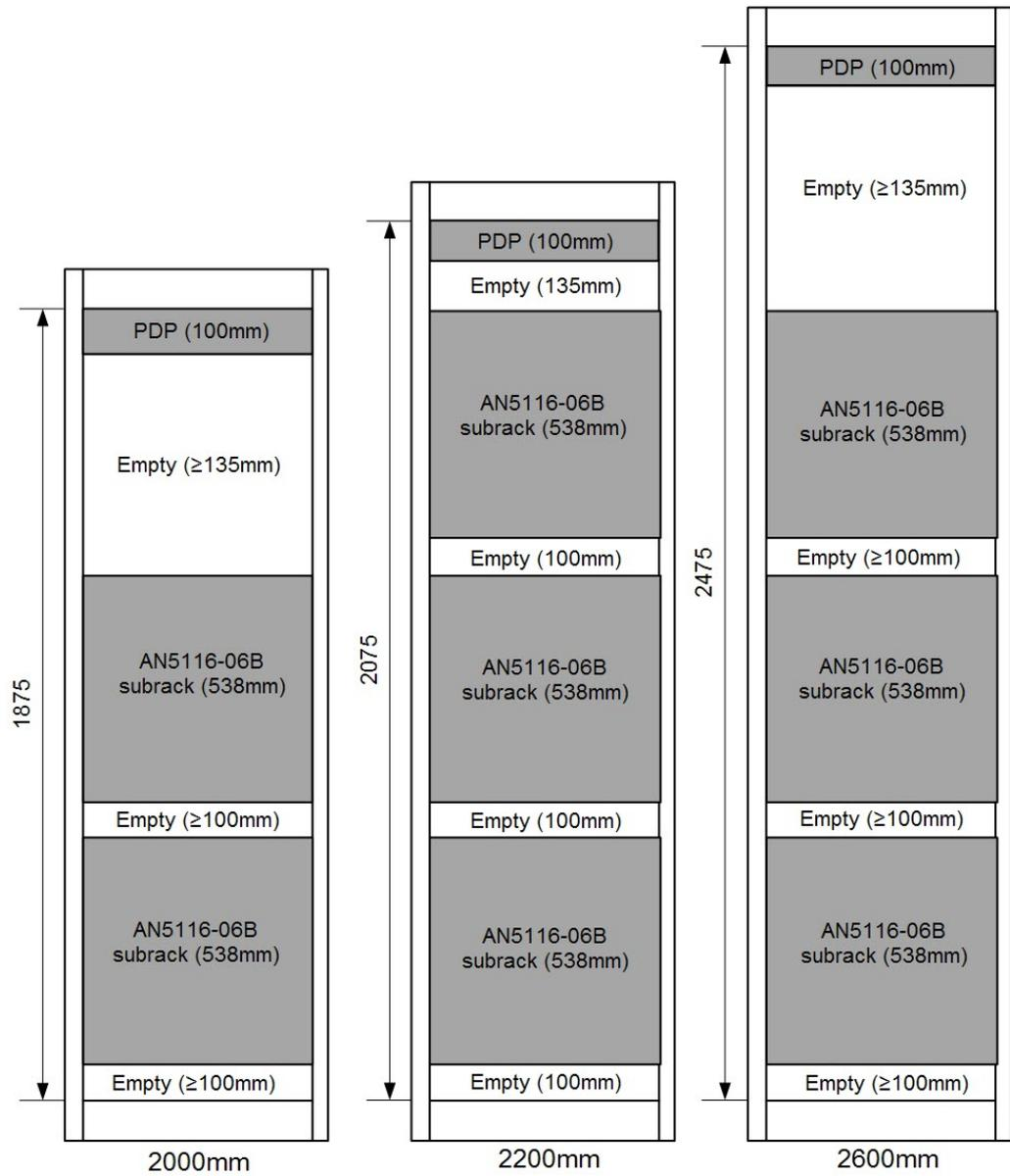
Figure 2-11 The layout of the 21-inch cabinet
