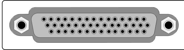
Figure 7-23 The pins of the DB-44P connector
