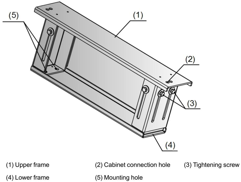
Figure B -1 The adjustable cabinet base (type I, II and III)
