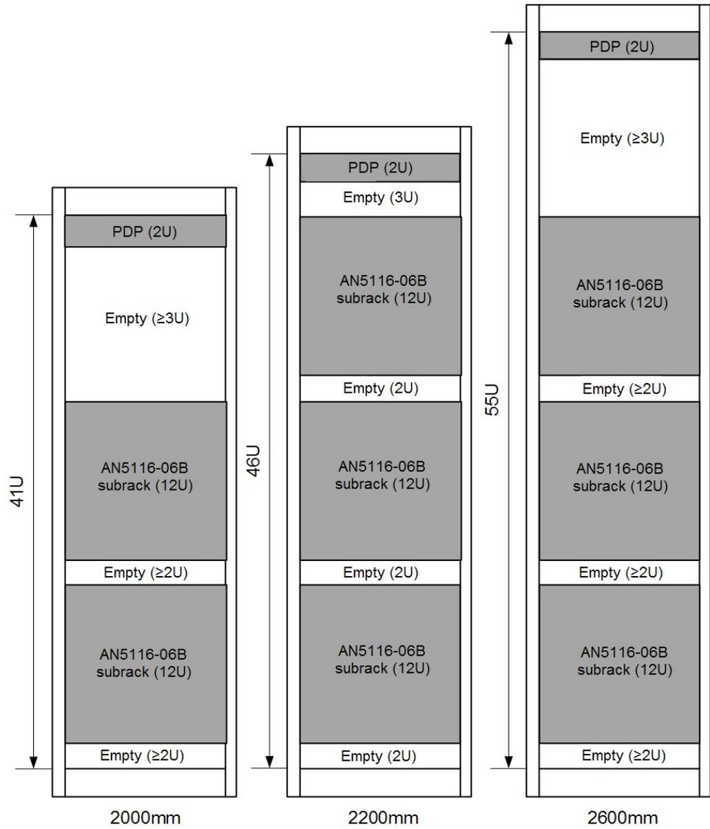
Figure 2-10 The layout of the 19-inch cabinet
