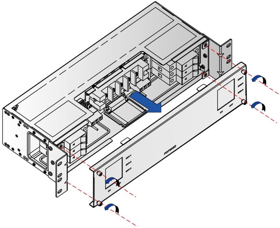
Figure 7-7 Removing the PDP's front panel
