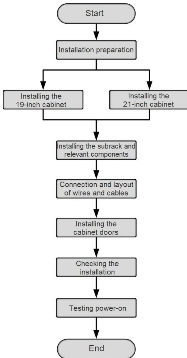
Figure 3-1 The equipment installation flow
