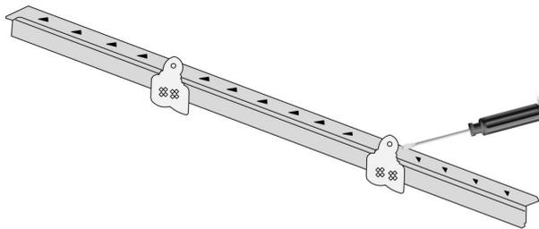
Figure 4-1 Prying the steel tab
