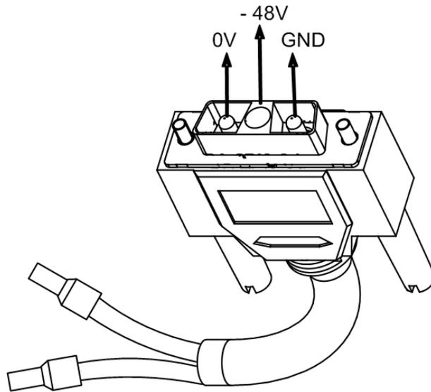
Figure 7-12 The subrack power cable
